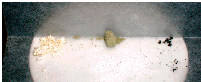
Figure 2. Powdered samples of the 1·3 cocrystal, before pressing (left), after pressing to 3 GPa in a multianvil press (center), and after pressing to 6 GPa (right).
